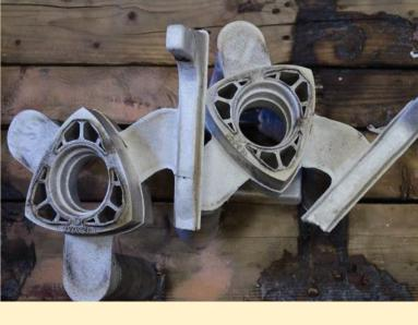
(b) Rotary engine rotor
